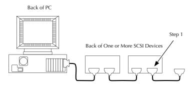
2. Attach the other end of the 50-pin to 50-pin SCSI cable to either of the identical SCSI ports on the back of the Scanner. Seat the connector firmly and pinch the wire clamps shut.
